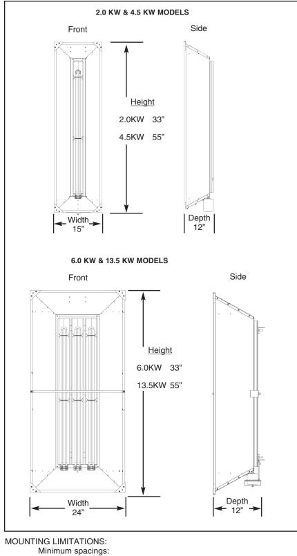
Ceiling to top of heater is 2 feet. Wall to sides of heater is 3 feet. Floor to bottom of heater is 10 feet. When used as a portable, a minimum of 7 feet to the front of the heater.
